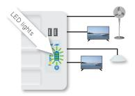
If all LED lights start blinking, too many "high consumption appliances" are connected to the system. The total consumption should not exceed 5.5 A.
