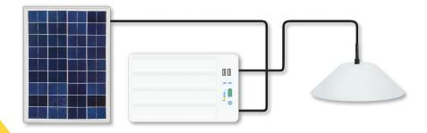
4 Connect the solar panel to the yellow socket of the LSHS. Connect the cable of the Fosera lamp to the blue socket of the LSHS.
