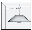
Place the lamp at your desired location and use the Hook Screw (F), which is included in your PSHS PAYG package. Make sure the cable is not pulled too tightly. If you need to extend the cable, please use a cable provided by fosera.
