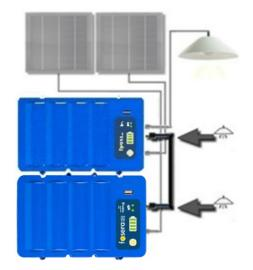
When more battery capacity is needed the fosera PSHS PAYG can be easily expanded:
