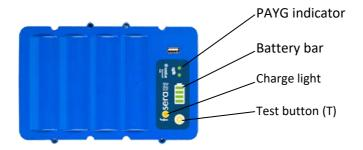
During the daytime the yellow charging light should be always on. It indicates that the system is being charged and is well connected to the module.
