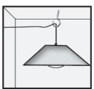
Place the lamp at your desired location and use the Hook Screw (E), which is included in your PSHSPAYG package. Make sure the cable is not pulled too tightly. If you need to extend the cable, please use a cable provided by fosera.
