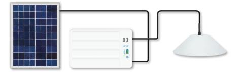
4 Connect the solar panel to the yellow socket of the PAYG LSHS. Connect the cable of the Fosera lamp to the blue socket of the LSHS.
